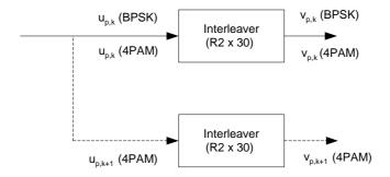
Figure 22A: Interleaver structure for E-DCH
